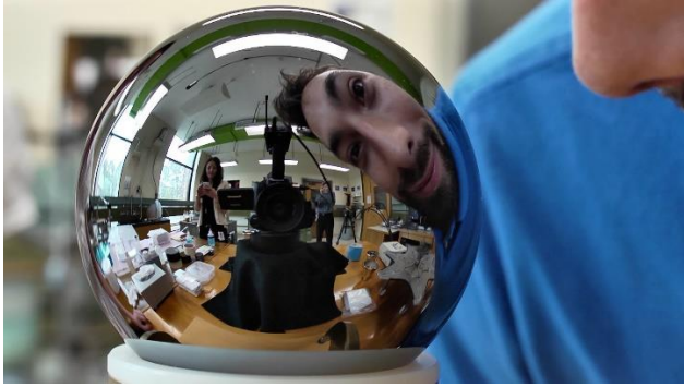
The world's roundest object, a sphere made of silicon 28.
