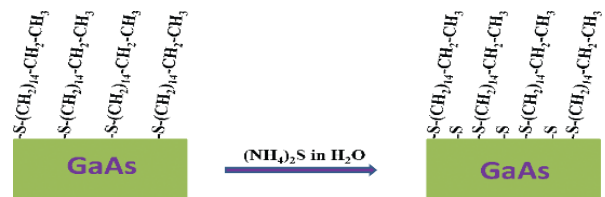
Fig. 2. Introduction of the additional step consisting of treatment of SAM coated GaAs samples in the ammonium sulfide solution. This hybrid approach allows increasing density of sulfur atoms reacting with Ga and As, which drastically increases photonic stability of such material in a biological environment.
