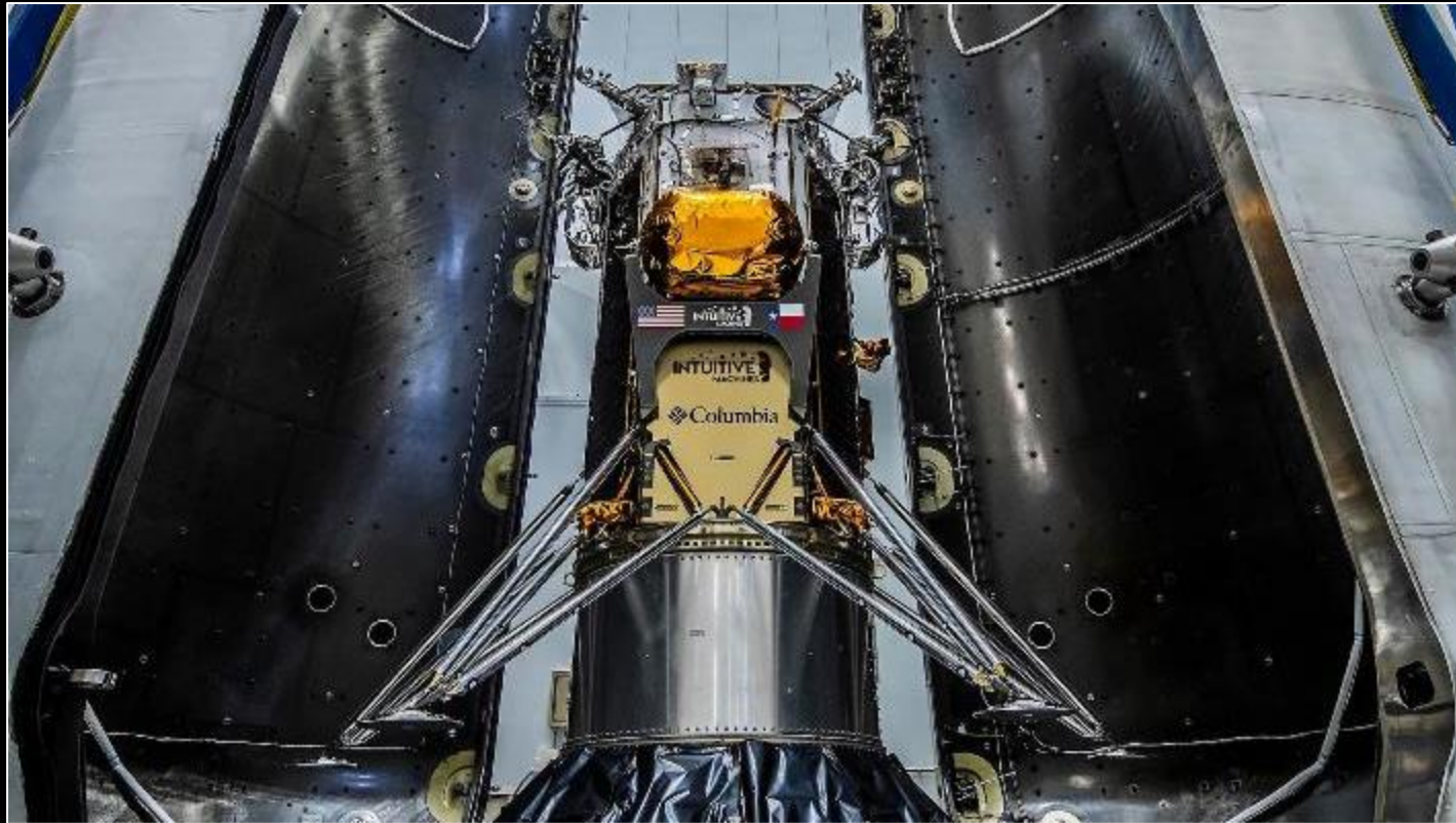
The Intuitive Machines' IM-1 lunar lander being readied to be housed inside a Falcon 9 fairing.
