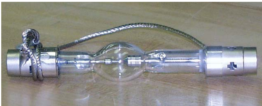
450-W xenon lamp, removed from the protective case.
