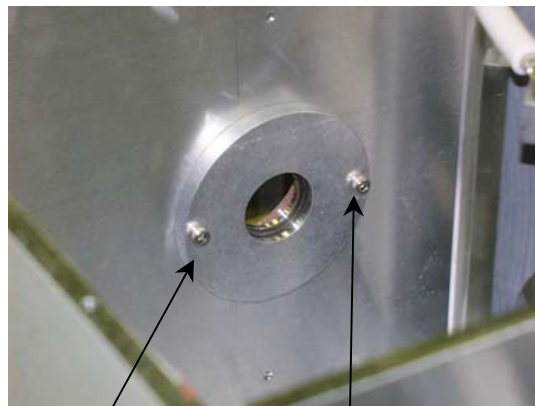
Cap screws on interior wall of lamp housing.
